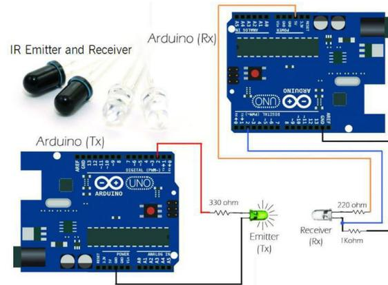
Error Free transmission was achieved in both One-Way and Two-Way transmission. With off the shelf LED is a communication distance of 22cms was observed. Using better grade LED's and Photodiodes can enable two-way communication to much greater distances.
